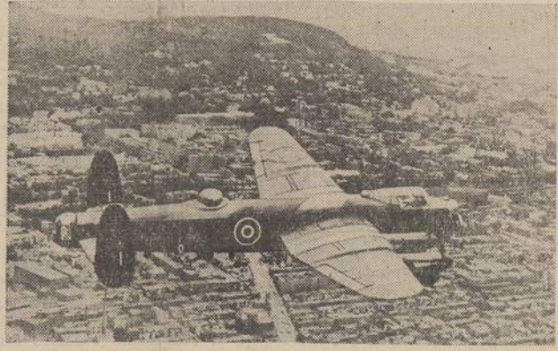
An excellent view of the Lancaster, first of England's mighty four-engined bombers, as it arrives at Dorval airport in Montreal, Canada. It will be demonstrated and then produced on Canada's assembly lines. This bomber can carry eight tons of bombs, has a top speed of 300 miles per hour and a range of 3,000 miles. It has ten machine guns.
