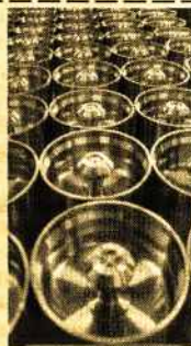
Manufactured parts for nuclear containers made in stainless steel.
